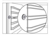
To re-insert, first hook the rail into place at the back (1) and then insert the front and press into place (2).
